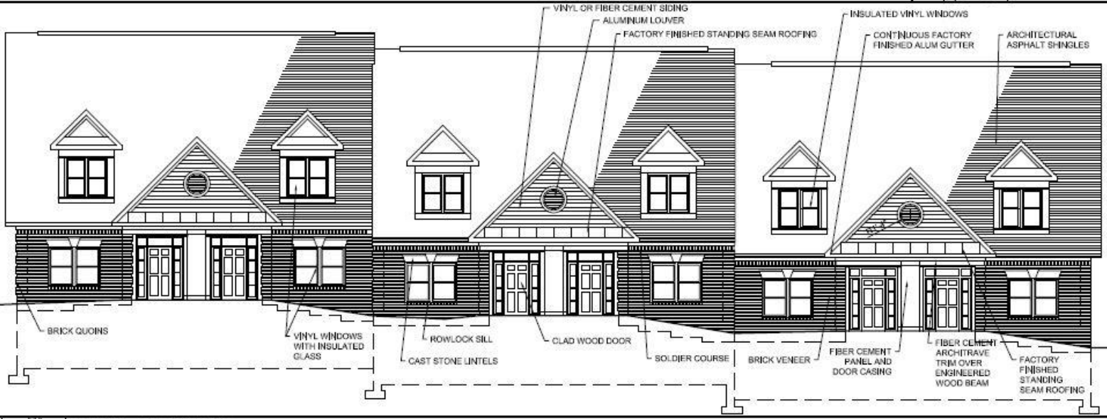
C2 1/8" = 1'-0" FRONT ELEVATION
